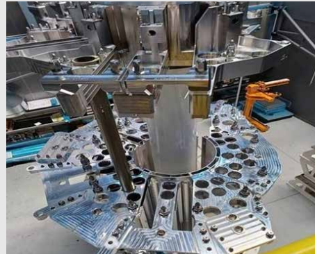
FACTORY ASSEMBLY OF THE RJH REFLECTOR
