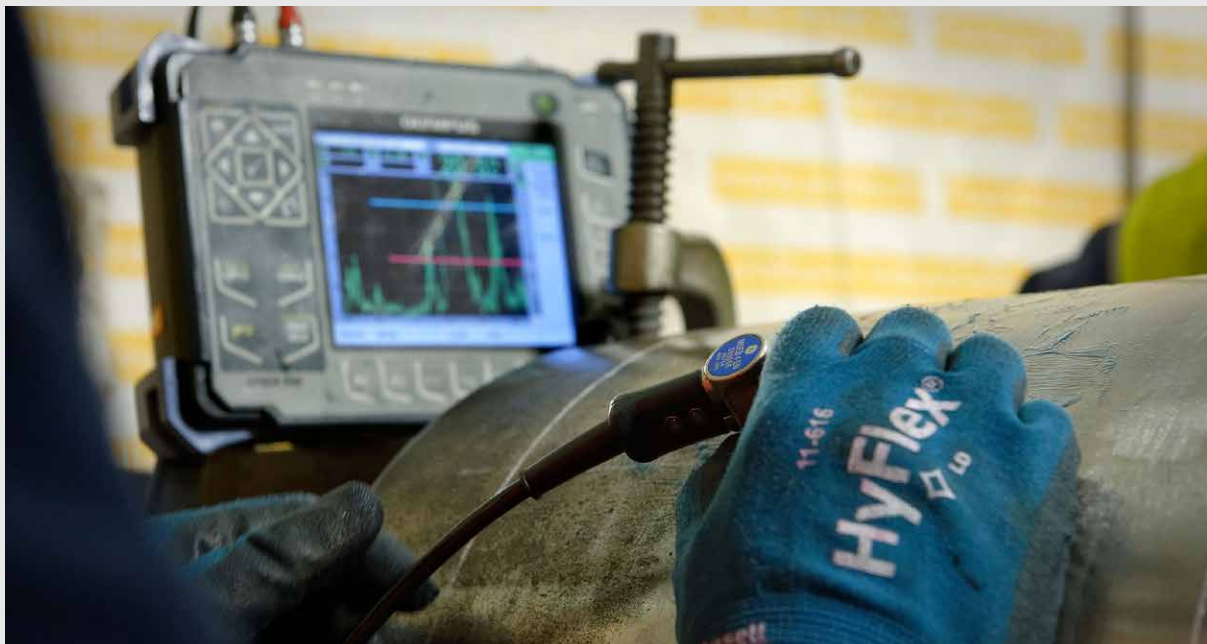
ULTRASONIC EXAMINATION OF WELDS
